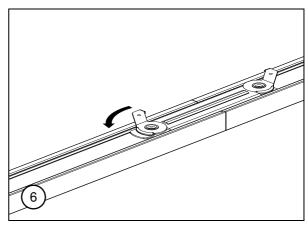
**Warning** | When installing tracks with Wave gliders the pilots must <u>not</u> be moved until fitted, moving the pilots & gliders when upside down can promote the glider cord getting tangled within the glider channel.
