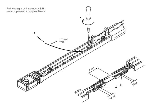
**NB** Once tested, tension wire can be cut, and raw end can be covered with heat shrink supplied. Warming the rubber with warm air will cause rubber to shrink and adhere to the wire.
