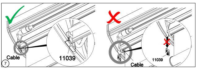
Locate cable back into corner cut-out. Re-locate spacer 11039 into place.
