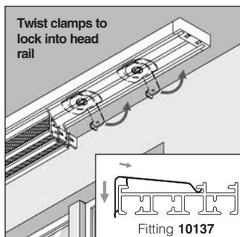
Twist clamps to lock into head rail
