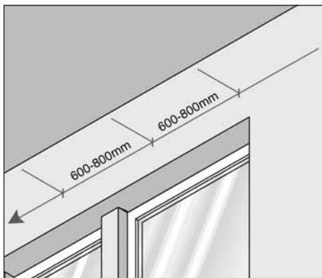
② Draw a straight line along the top of the wall where the track is to go and mark on this the position of the brackets. Each end bracket should be no more than 10cm from the ends of the track and each subsequent bracket should be spaced equally apart at 60-80cm intervals.
