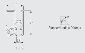
Due to the enclosed channels, this curtain track can be forward and reverse bent. The standard bending radius of 200mm can be reduced to as low as 100mm for reverse and forward bends if no overlap arm is used.
